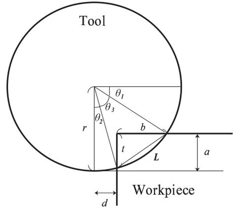
**FIGURE 7.** Machining model of slit collar
