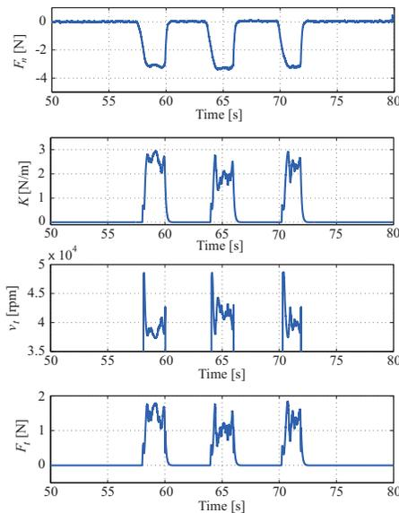
**FIGURE 8.** Experimental result of estimation hand stiffness of grinding force control
