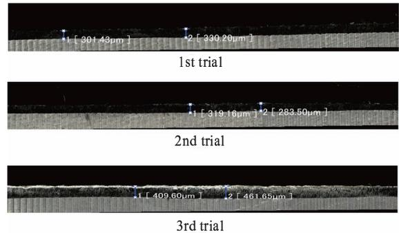
FIGURE 13. Machining surface with grinding force control machining
