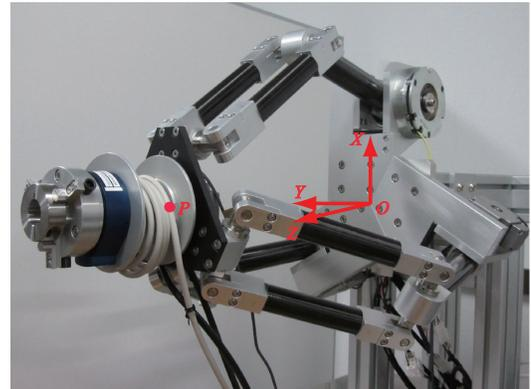
FIGURE 1. Machining support system with parallel link mechanism
