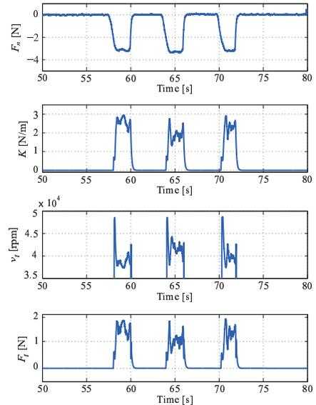
FIGURE 12. Experiment result with grinding force control
