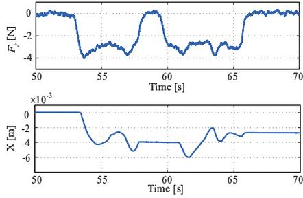
**FIGURE 5.** Force and end effector position of hand stiffness estimation experiment
