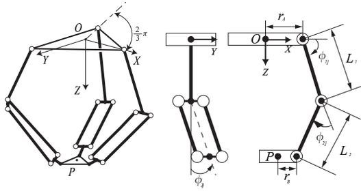
FIGURE 2. Kinematic parameters of DELTA
